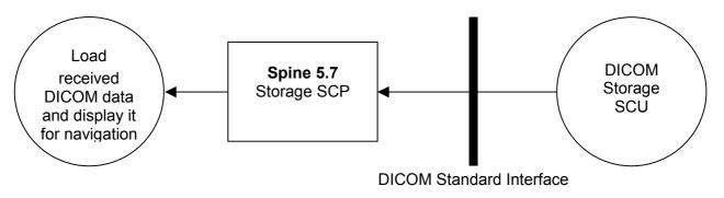
Figure 4-1: Application Data Flow Diagram
