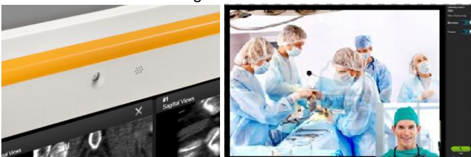
Figure 10: Brainlab Buzz video conferencing. The video conferencing camera and microphone are integrated into the touch display frame
