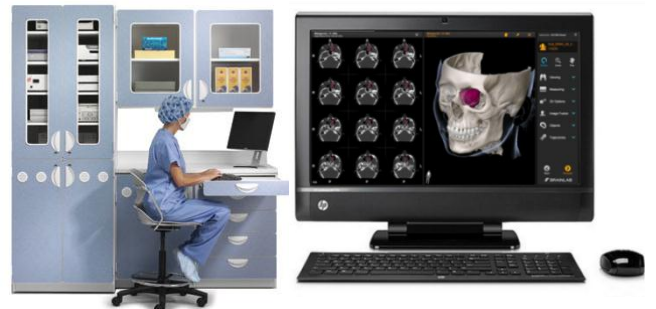
Figure 7: Integration of Nurse PC in the OR integration system. The Nurse can take over control but can also push content to the workstation (e.g. DICOM Viewer). Documentation functionality can be controlled from nurse PC.
