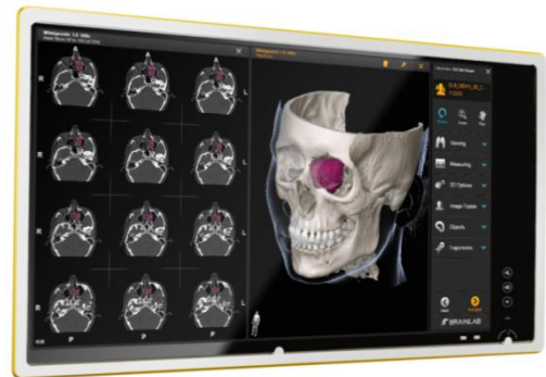
Figure 13: Brainlab Buzz with interactive DICOM viewer. The display shows images from a CT scan: a series of single layers on the left and an on-the-fly calculated 3D visualization of the data on the right. Objects can be highlighted for further planning. In this example, an object (a tumor in red) has already been defined and displayed in a 3D view.
